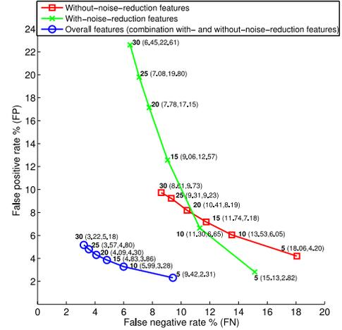
Fig. 12. Detection error tradeoff (DET) curve for various feature sets for the WMFPR, where the value of  $c_{\text{nonpattern}}$  was fixed at 1 to determine an optimum value of  $c_{\text{pattern}}$  in the SVM. The bold annotation represents the value of  $c_{\text{pattern}}$ . The overall features achieved the optimal curve in the DET plot.
