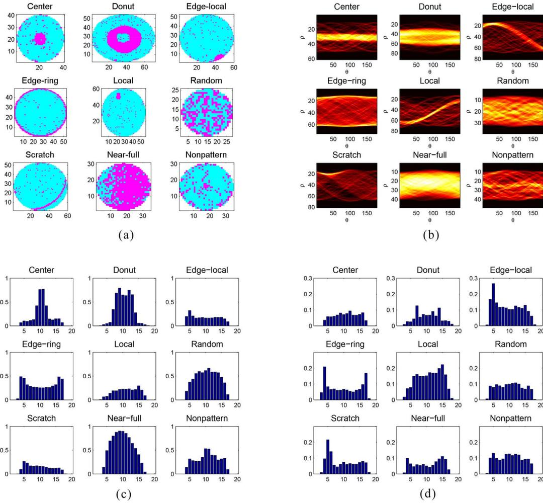
Fig. 2. (a) Typical examples of wafer map failure types. (b) Projection results  $\mathbf{G}$  following the Radon transform. (c) Radon-based features  $\mathbf{R}_\mu$ . (d) Radon-based features  $\mathbf{R}_\sigma$ .
