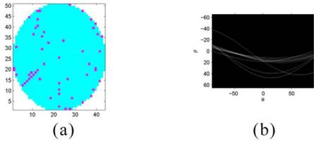
Fig. 4. Example of line detection by using the Hough transform. (a) Scratch wafer map. (b) Result of the Hough transform for (a). Accumulator  $\mathbf{A}$  has local maxima at approximately  $(\rho, \theta) = (-1, -45)$ , which indicates the line segment in (a).
